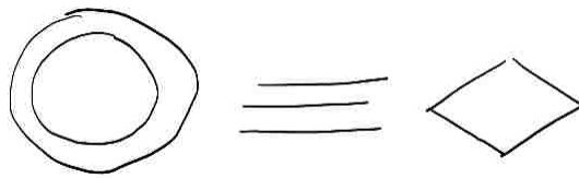
Figure 4.2: Examples of symbols composed of geometric shapes. A finite state machine’s Accept State symbol, a bond diagram’s Triple Bond symbol, and a flowchart’s Decision symbol.
